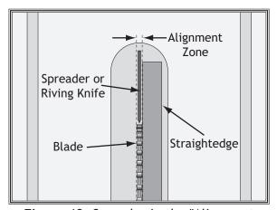
**Figure 40.** Spreader in the "Alignment Zone."
